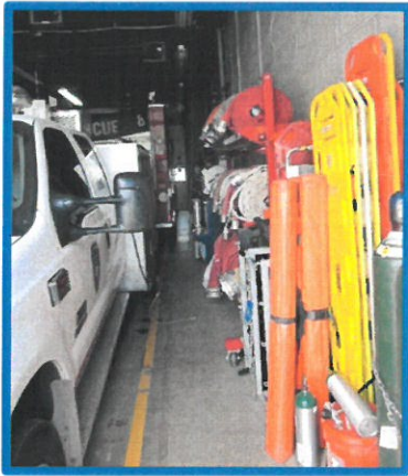
Figure 4-3 (left): Storage of spare hose, equipment, tools, and even SCBA is crowded into the apparatus bays. Figure 4-4 (right): Firefighter PPE is stored in racks in the apparatus bays, which is not recommended as it is exposed to UV light and vehicle exhaust emissions fumes and particles.
