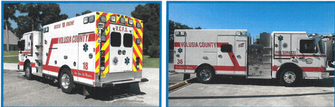
Figures 4-31 and 4-32: Front and rear views of combination fire pumper/rescue/ambulance unit utilized by Volusia County, Florida. Note: Volusia County will probably purchase four door units the next time to provide one additional riding position and additional equipment storage space.
