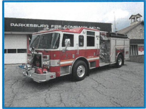
Figure 4-17: Engine 8-2; 2001 Pierce pumper 2000 GPM pump capacity; 750 gallon water tank 50 gallons Class A foam; 30 gallons Class B foam Very good condition Assigned to Parkesburg/Central station
