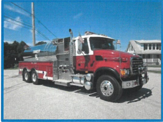
Figure 4-20: Tanker 8; 2006 Mack/4 Guys tanker/pumper 1500 GPM pump capacity; 3200 gallon water tank Very good condition Assigned to Pomeroy/East station
