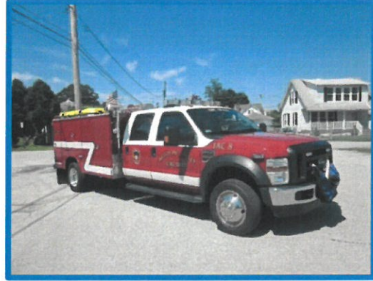
Figure 4-21: TAC 8; 2009 Ford Mini-pumper; 300 GPM skid pump capacity; 200 gallon water tank Rescue tools Excellent condition Assigned to Pomeroy station
