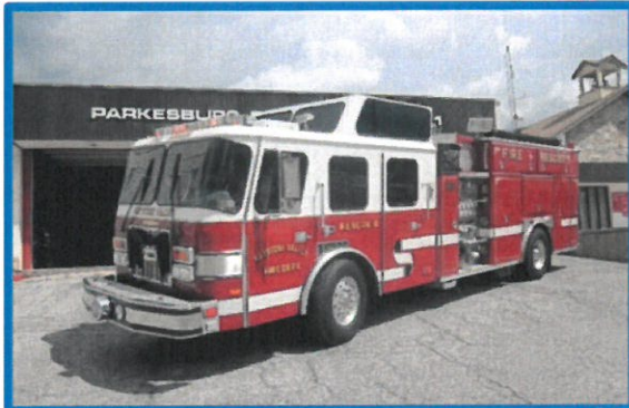
Figure 4-18: Rescue 8; 1994 E-One pumper 1500 GPM pump capacity; 750 gallon water tank; rescue tools Fair condition Assigned to Parkesburg/Central station
