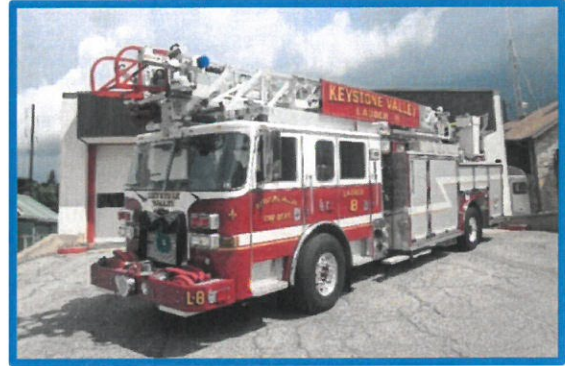
Figure 4-19: Ladder 8; 2012 Pierce Quint 1500 GPM pump capacity; 480 gallon water tank 75' aerial ladder Excellent condition Assigned to Parkesburg/Central station
