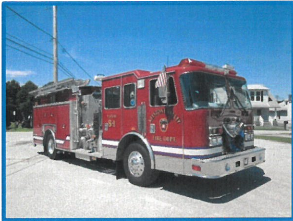
Figure 4-16: Engine 8-1; 1999 KME pumper 1250 GPM pump capacity; 750 gallon water tank; 50 gallons Class A foam; rescue tools Good condition Assigned to Pomeroy/East station
