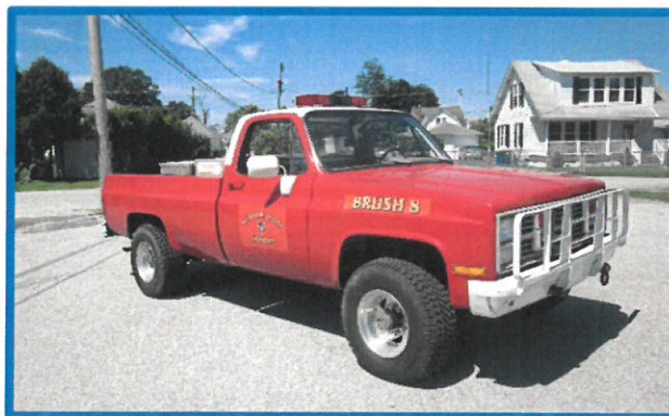
Figure 4-28: Brush 8; 1984 Chevrolet 4x4 brush truck 125 GPM skid pump capacity; 200 gallon water tank Owned by Pennsylvania Department of Natural Resources Poor condition (removed from service during study) Assigned to Pomeroy/East station
